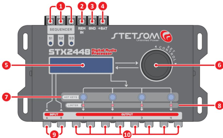
**1. SEQUENCER:** It allows sequential activation of other products through the remote activation (REM) connection. Use a cable of at least **AWG 18**.
