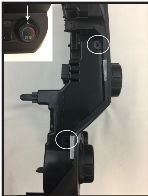
4. Make sure that the white line on the temperature control knob is centered at the top. Remove back of factory dash panel by releasing the locking tabs on each side.
