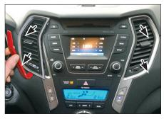
2. Unclip air vents at left and right side
