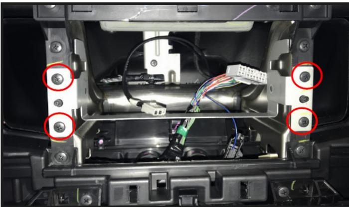
With the main fascia panel out of the way, undo the following four screws and put these to one side. With the screws out, fully remove the metal bracket.
