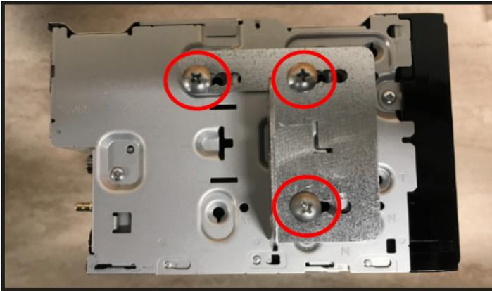
Take the brackets found within the kit and offer them up to the relevant side of the new radio. Once positioned correctly, screw them into place using a set of radio screws (*not supplied with this kit*).
