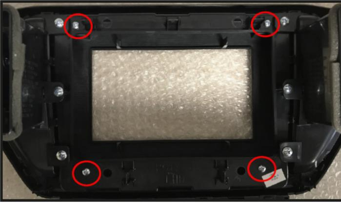
Position the new fascia panel in front of the main air vent/trim panel and screw into place using the screws provided in this kit.
