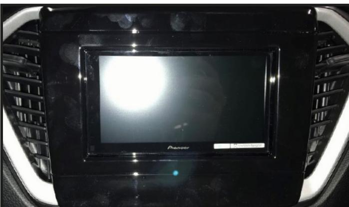
Place the new fascia panel over the front of the new radio to complete the installation.
