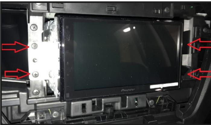
With the brackets attached and the connections made to the rear of the radio, place the unit into the dashboard and screw into place using the four pre-existing screws removed in earlier (*see Step 2*).
