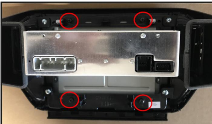
Undo all four screws located on the rear of the main fascia panel. These screws will disengage the air vents and trim from the main single DIN unit/touch screen.
