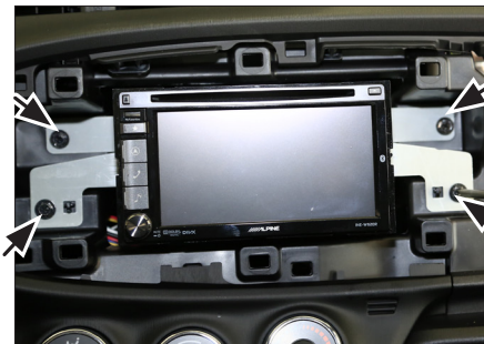
8. Connect all required circuit points Place Double DIN head unit on dash board Fix double DIN head unit with 4 OEM screws
