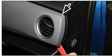
2. Unclip plastic panel - start from the right side
