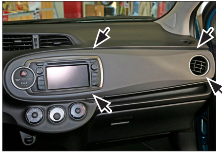
2. Unclip plastic panel - start from the right side
