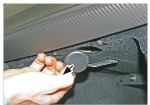
Open the glovebox and begin by uncliping the following circular piece of plastic.
