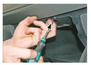
Once the circular cap has been removed, proceed to undo the screw that is located therein.
