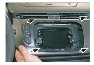
With all of the screws removed, use a panel removal tool to disengage the main fascia panel and remove it whilst disconnecting the side button connector(s).
