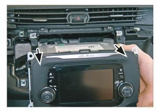
With the screws removed, begin to pull the radio out of the dashboard and disconnect all of the wiring.
