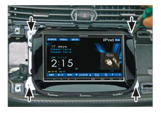
With kit assembly performed correctly, make all of the connections to the stereo and install into the dashboard. Once seated correctly, secure the unit by using the pre-existing screws.
