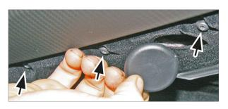
Proceed to then remove the following screws that are on show within the lip of the glovebox.
