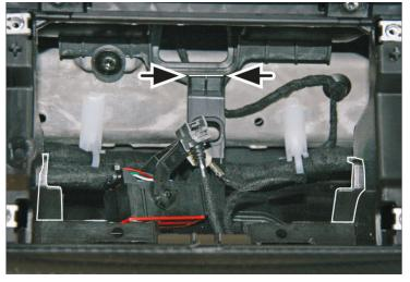
The highlighted area(s) will need to be cut out of the dashboard in order to allow the new double DIN unit to sit correctly.
