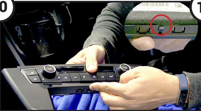
Relocate the climate control button panel into the new double DIN fascia panel, ensuring that the middle clip is lined up for a perfect fit
