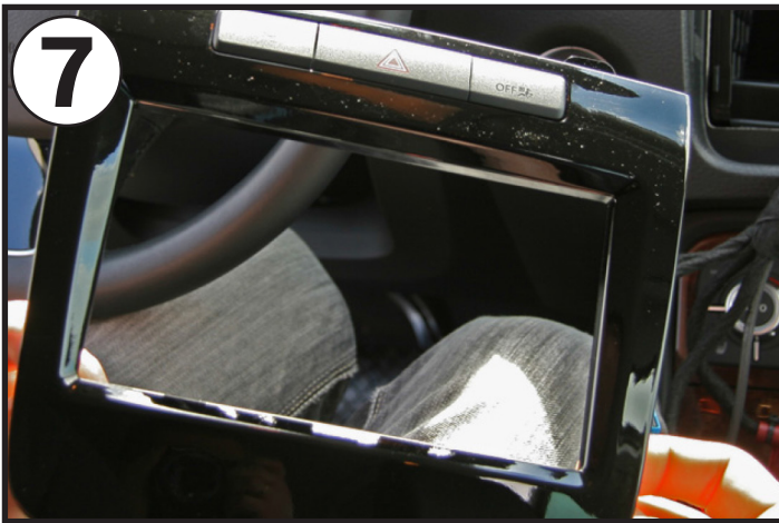
7 Push the button panel from the OEM panel into the new fascia panel
