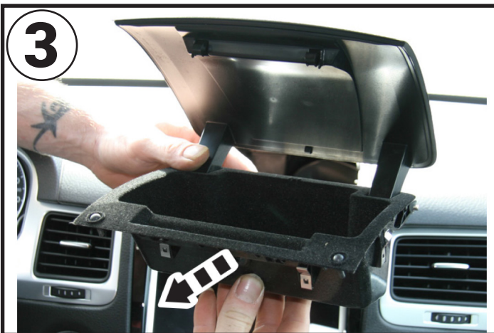
3 With the screw removed, the entire upper tray can now be removed from the dashboard
