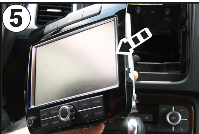
5 With the screws removed, the entire OEM head unit and panel can now be removed from the vehicle. Ensure all wiring to the OEM head unit is disconnected
