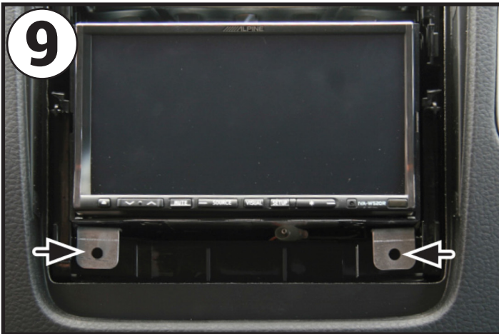
9 Make all required connections to the new head unit and push it into the dash. Secure it in place using screws at the points highlighted by the arrows.
