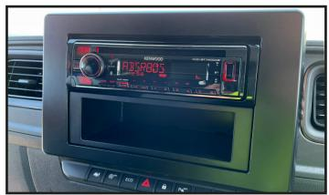
Insert the radio cage into the empty portion of the fascia and install the fascia onto the dashboard. You can then fully connect the radio.
