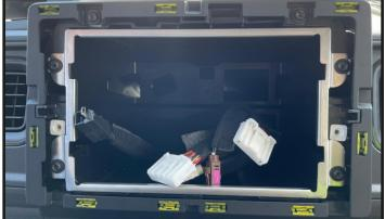
Using the 4x pre-existing screws from the main head unit, screw the frame bracket into place.
