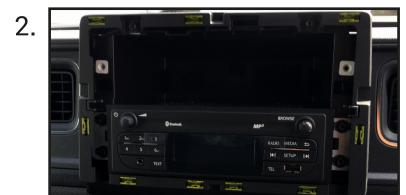
With the trim out of the way, undo the 4x screws that surround the main head unit and remove it whilst disconnecting all of the wiring.
