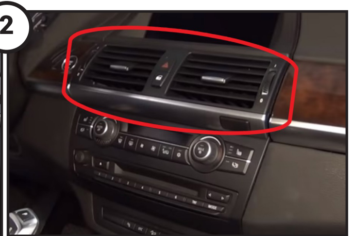
Use a panel removal tool to remove the air vents (circled).
