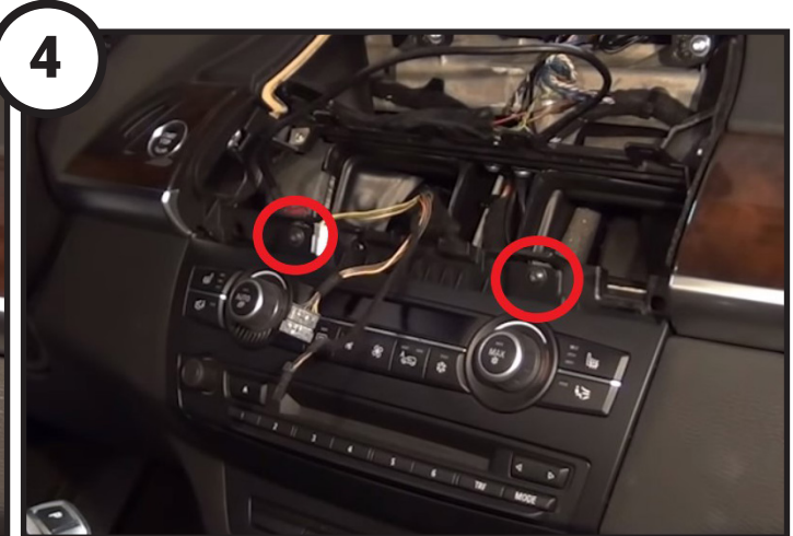
Remove the two screws securing the lower fascia panel
