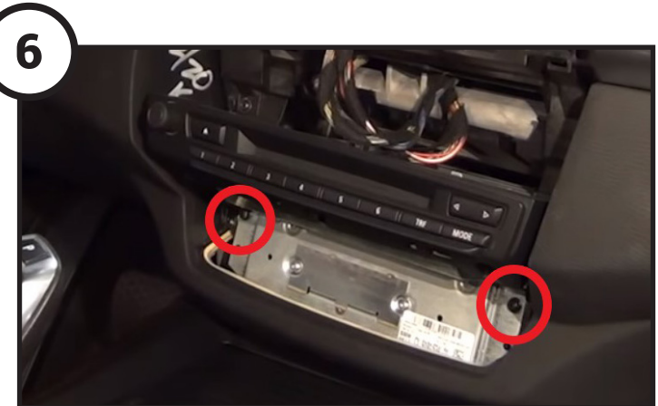
Remove the two screws securing the OEM head unit in place. Disconnect and remove the head unit.
