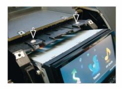
**19**. Spare OEM hazard light switch by Ford required. Ford part No: 1519127. Fix this into the facia plate.
