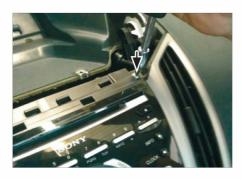
13. Remove screws from OEM head unit
