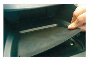
**2.** Carefully unclip and remove speaker grill on top of dashboard
