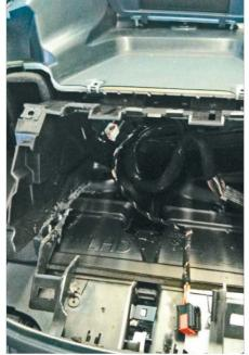
**12.** Unclip and remove air vents
