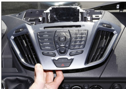
4. Remove OEM head unit by pulling it towards your direction
