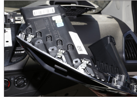
5. Unclip air vents from OEM panel
