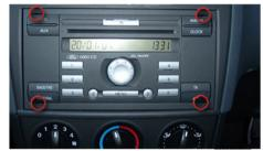
Remove the original radio using Ford radio release keys.
