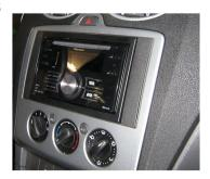
Fit the head unit into the cage, then fit the replacement panels.
