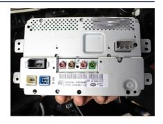
14. Attach the included brackets to either side of the aftermarket head unit and place into the dash.
