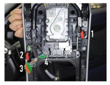
6. Remove the side panel using a panel removal tool.
