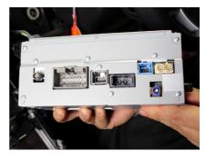
12. Remove all 4x screws surrounding the vehicle display.
