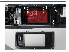
10. Remove the 2x screws on either side of the head unit.
