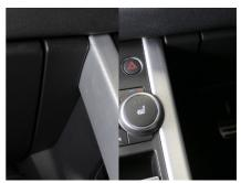
3. There are 2x T-20 screws located underneath the front arch of the centre console. Remove these screws.
