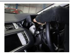
2. Remove both side trims on either side of the centre console with a panel removal tool.
