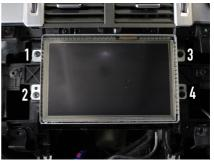
13. Disconnect all wiring from the vehicle display.
