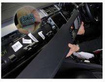
9. Remove the 6x screws surrounding the pre-existing button panel and replace it with the new fasica panel.
