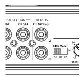
**Note:** The preamp output signal is not affected by the amplifier's filter controls. If the input signal is full-range, the preamp output will be full-range.
