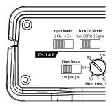
If you wish to send four discrete channels into the JD400/4, simply use all four inputs and set the "Input Mode" switch in the "4 Ch." position.
