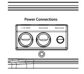
The JD400/4's "+12 VDC" and "Ground" connections are designed to accept 4 AWG power wire. 4 AWG copper wire is a minimum power wire size for this amplifier.
